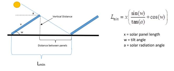
1. Determine  $L_{min}$  for the Solar Panels.
